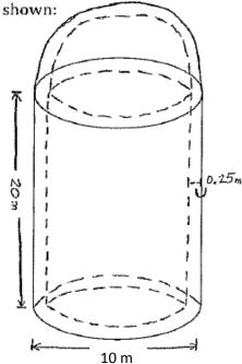
1. The <u>inside</u> diameter of the cylinder and spheres is needed to calculate the volume. You must determine the <u>diameter</u> of the inside of the silo, if the walls are 0.25m thick.
