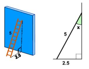
A 5-foot ladder leans against a wall. What is the angle between the ladder and the wall?
